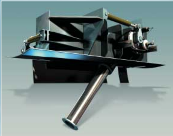
kMAG Rotor – Magnus Effect Rotary Stabilizers (retractable version)
